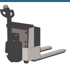
**Electric pallet jacks** make quick work of moving loads around the workplace. Pallet jacks protect your back from strains and injuries by moving heavy and awkward loads and objects that would be unsafe to lift manually.
