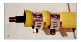
Crimping Type Compressed Air Clamps Approved for Use
