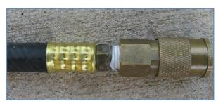
Compressed Air Hose with Crows-foot Connectors (see retainer pin)
